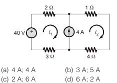
**Q.28** The currents  $I_1$  and  $I_2$  in the below circuit are respectively
