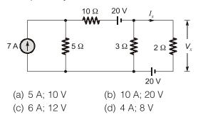
**Q.30** For the circuit shown in figure below, the value of current, *I* is
