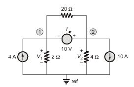
Let current through 10 V source is *I*. Applying KCL at node 1,
