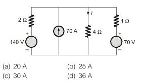
Q.19 For the network shown in the figure below, what is the voltage across the current source?
