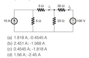
**Q.29** The currents  $I_x$  and  $V_x$  in the below circuit are respectively
